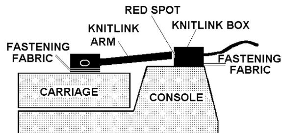
5. When positioned correctly, remove the backing strip of the fastening fabric from the base of the KnitLink Arm and fix to the carriage. Remove the backing strip of the fastening fabric from the base of the KnitLink Box and fix to the console.
